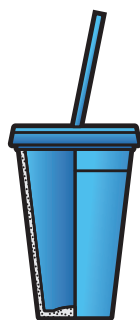
Air Insulation Air between inner & outer walls.
